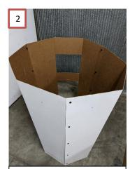
Fold all 9 sides of the bolted structure to form a cone shape. Connect the final seam with 5 more bolts to secure the shape.
