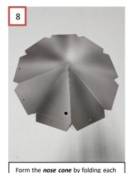
side and connecting the main seam
