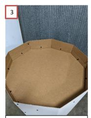
With the structure upside down (wide end facing up), insert the nonagon-shaped *floor panel* as shown and connect with 9 bolts around the perimeter.
