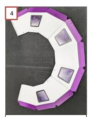
Lay out the upper *cockpit window* pieces as shown and bolt the rear seams together. See next step for detail.
