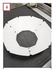
Gently fold each side of the *cockpit* windows and connect the third seam with 2 bolts to complete the ring shape.
