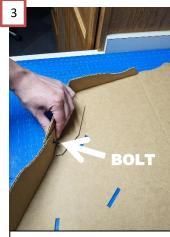
Locate the **ROCK BED** piece and flip it over. Fold up all of the edges along the front and connect them with bolts as shown.
